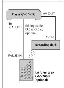
Using the RM-V704U/V700U remote control, it is also possible to perform deck-to-deck Random Assemble Editing. The playback deck must be an R.A. Edit-capable IVC VCR. The recording deck can be...
